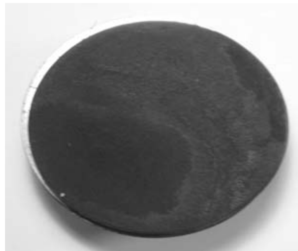
Fig. 6. Si engine piston head with TBC after thermal fatigue test
