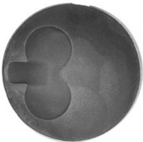
Fig. 5. Piston head of diesel engine with TBC after test
